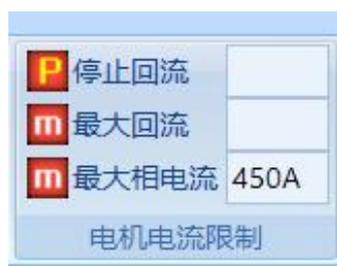
For the electronic brake function, when braking, the vehicle gives a braking electronic brake will be used to stop the return current, and the brake current does not exceed the maximum return value.
