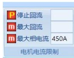
For the electronic brake function, when braking, the vehicle gives a braking signal to the controller, and the controller detects the brake After the signal, the electronic brake will be used to stop the return current, and the brake current does not exceed the maximum return value.
