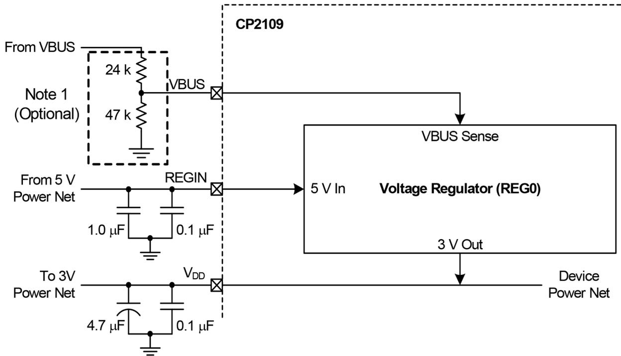
Note 1 : For self-powered systems where VDD or REGIN may be unpowered when VBUS is connected to 5 V, a resistor divider (or functionally-equivalent circuit) on VBUS is required to meet the absolute maximum voltage on VBUS specification in the Electrical Characteristics section.
