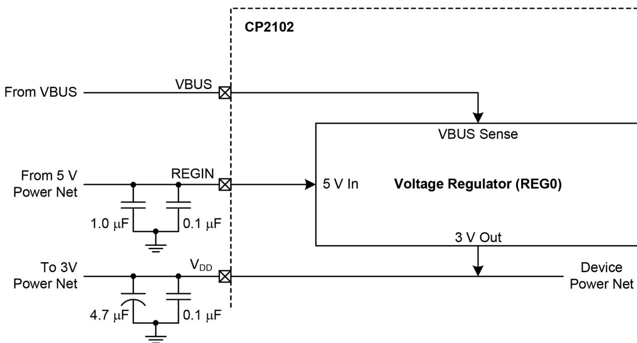
**Figure 7. CP2102 Configuration 2: USB Self-Powered**
