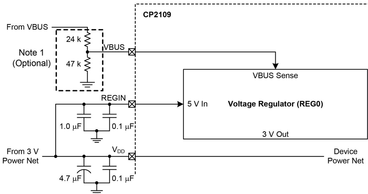
Note 1 : For self-powered systems where VDD or REGIN may be unpowered when VBUS is connected to 5 V, a resistor divider (or functionally-equivalent circuit) on VBUS is required to meet the absolute maximum voltage on VBUS specification in the Electrical Characteristics section.
