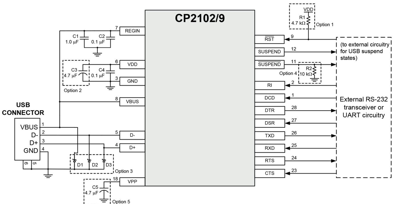
Option 1: A 4.7 k $\Omega$  pull-up resistor can be added to increase noise immunity.
