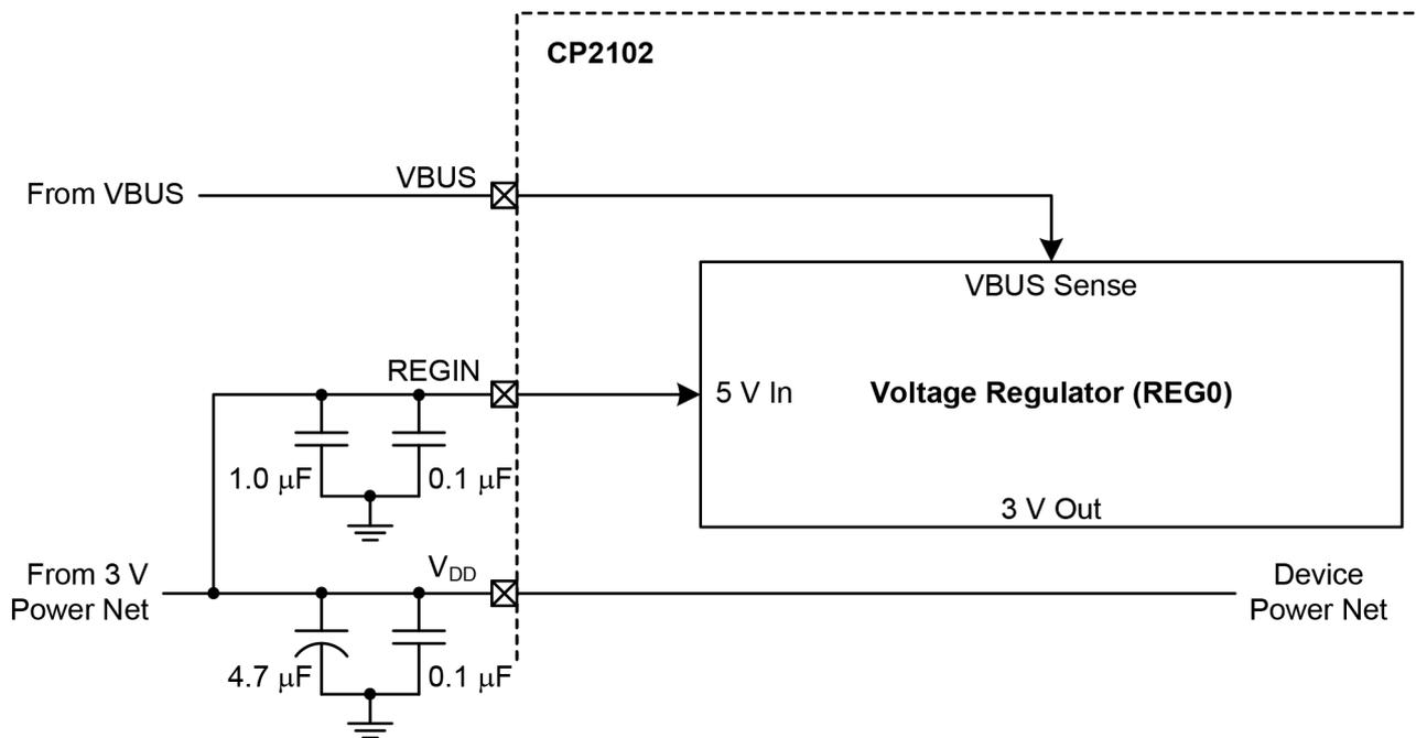
Figure 9. CP2102 Configuration 3: USB Self-Powered, Regulator Bypassed
